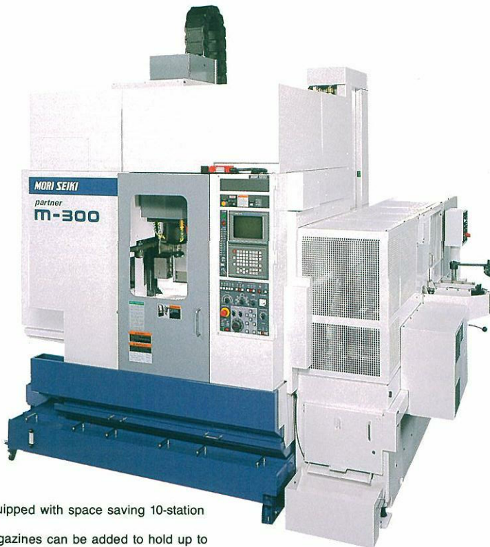
APC with a unique pitch transfer system makes possible the prompt replacement of workpieces. (M-300A2)
