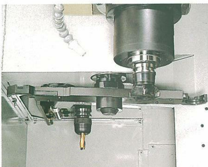
Standard-equipped with 20 tools, the ATC has a simple cam mechanism and assures high-speed tool change.
